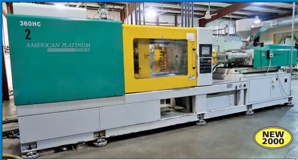
400 Ton x 39 Oz. Asian Pacific Machinery Model SM360HC Hydraulic Clamp PIMM
